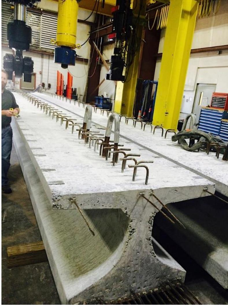
Figure 4.7: FIB-36 beams as delivered
