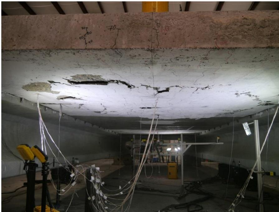
Figure 5.89: Load Case F2 – Failure at bottom of slab
