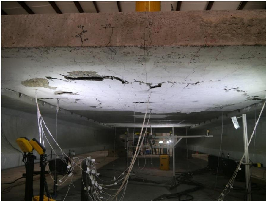
Figure 5.89: Load Case F2 – Failure at bottom of slab
