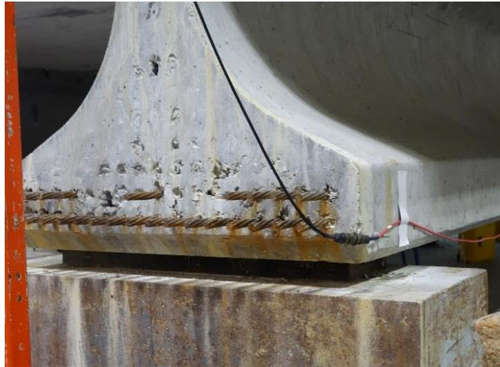
Figure 4.10: Bearing pad in place
