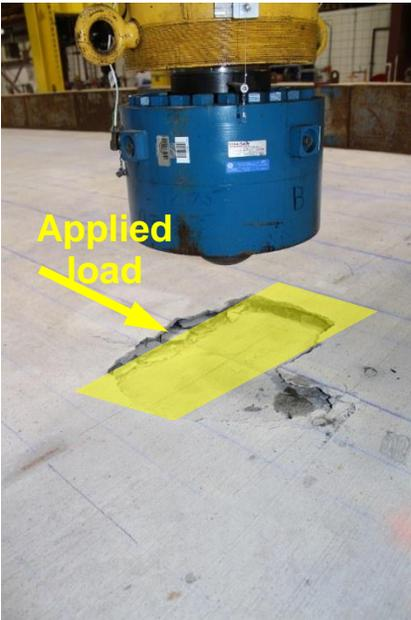
Figure 5.91: Load Case F3 – Failure at load point
