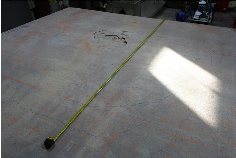
Figure 5.84: Load Case F2 – Tracing cracks at top of slab
