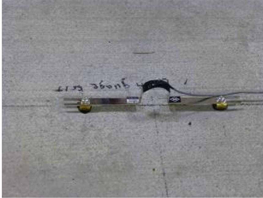
Figure 4.27: Typical full-bridge crack gauge
