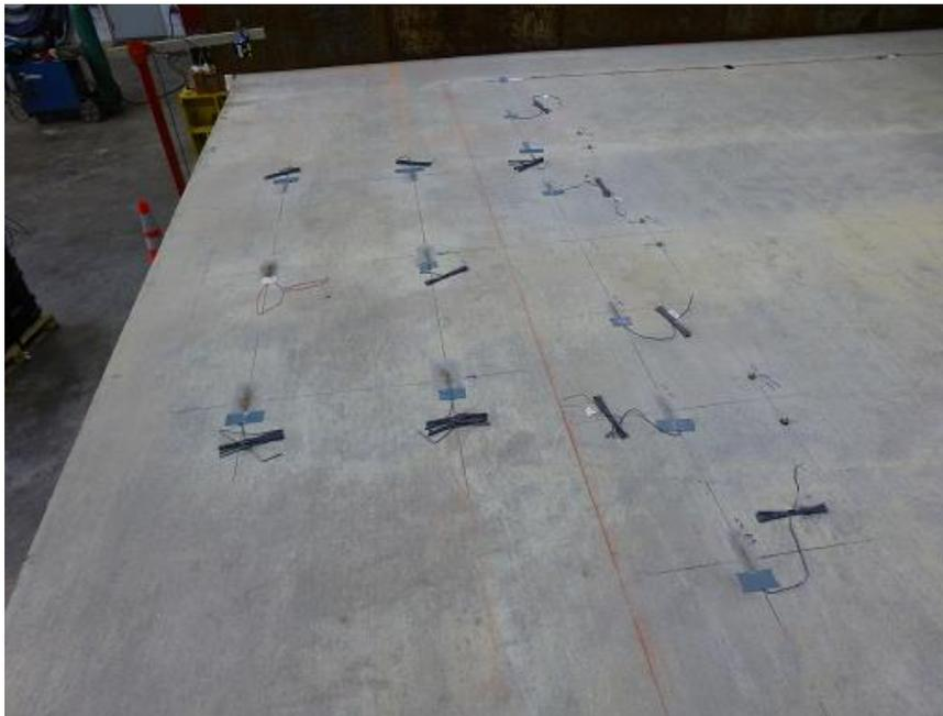
Figure 4.28: S2/F2 surface strain gauges
