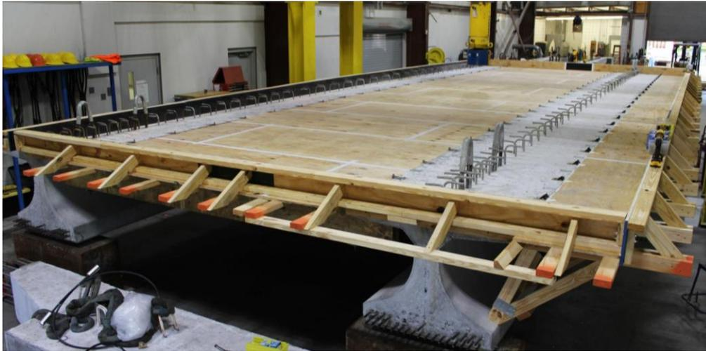
Figure 4.17: Overall completed formwork
