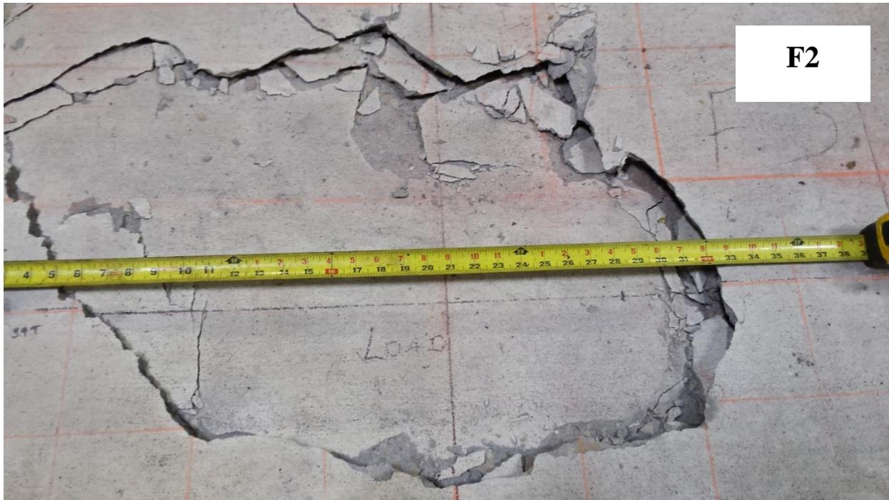
Figure 5.88: Load Case F2 – Close-up of failure at top of slab under load point
