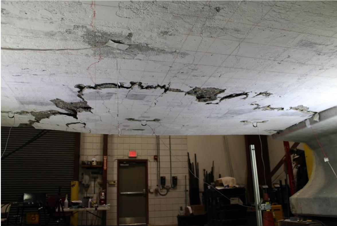
Figure 5.96: Load Case F4 – Extent of failure surface at bottom of slab
