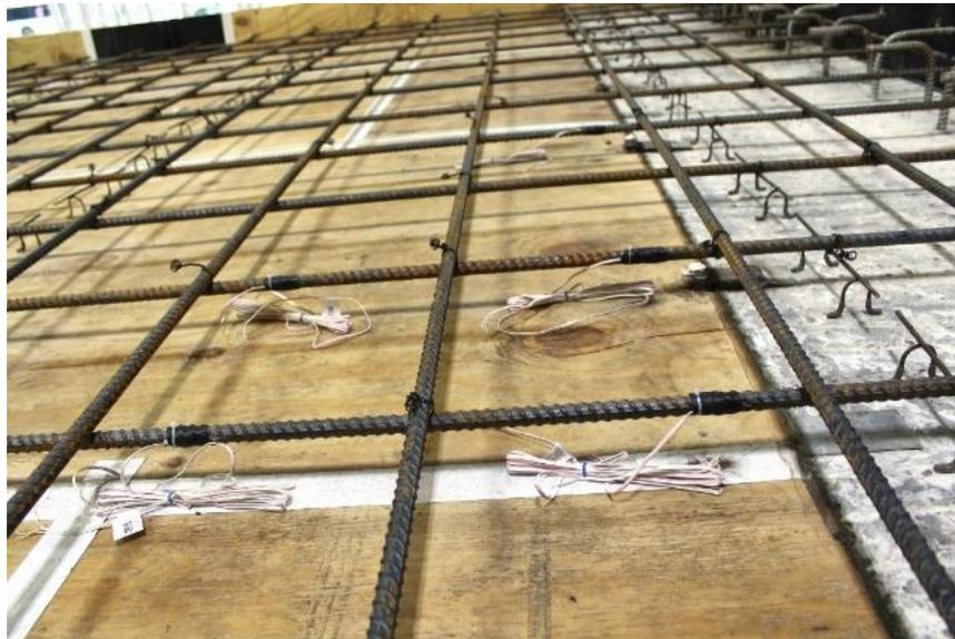
Figure 4.26: Strain gauges on bottom mat reinforcement
