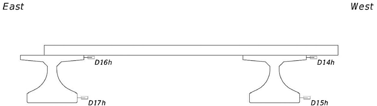
Figure 4.32: Horizontal girder displacement transducers
