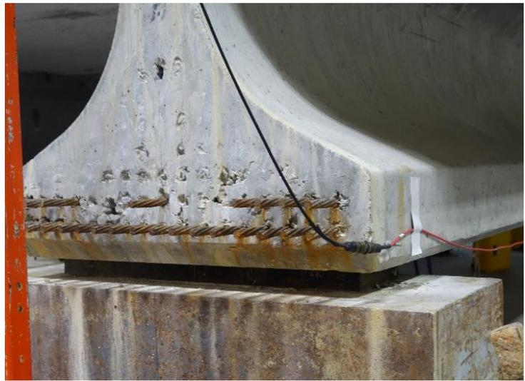
Figure 4.10: Bearing pad in place
