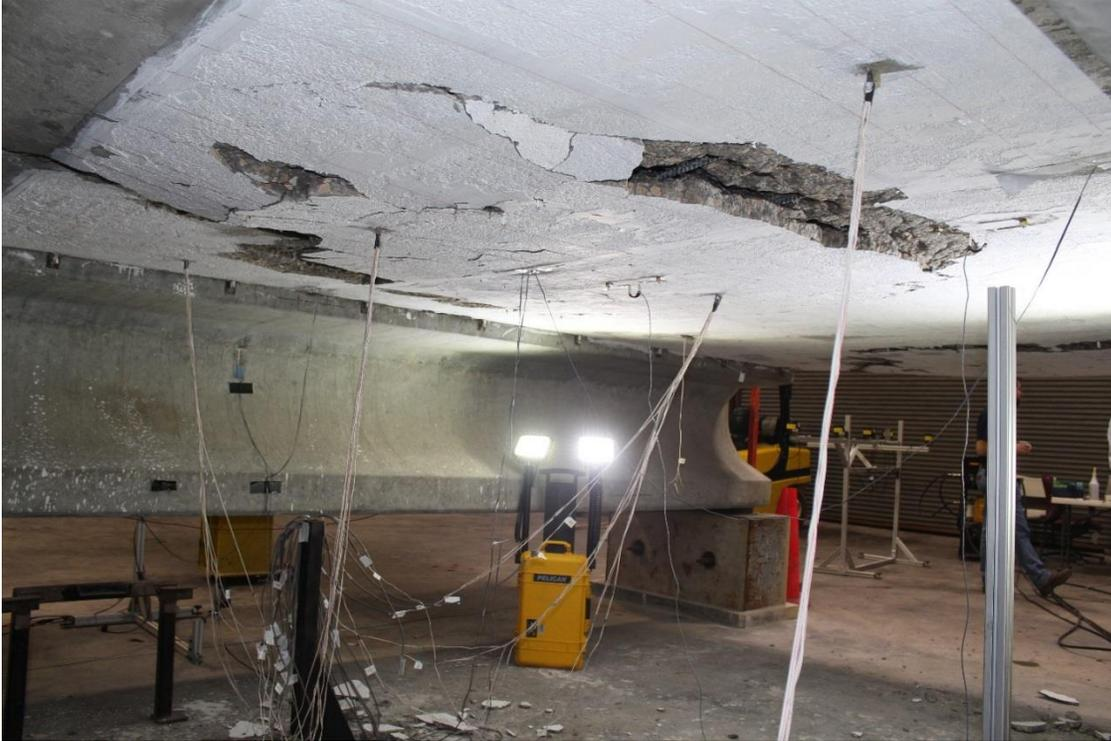
Figure 5.92: Load Case F3 – Extent of failure surface at bottom of slab
