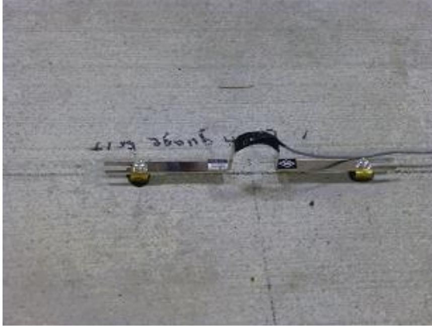
Figure 4.27: Typical full-bridge crack gauge
