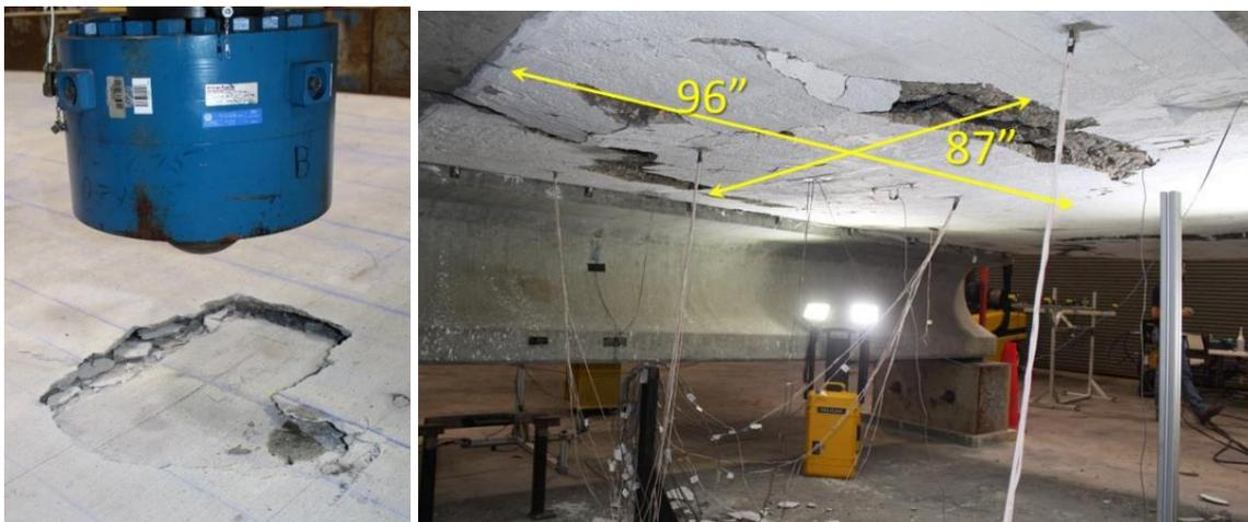
Figure 6.7: Top and bottom slab crack distribution and failure (F1-test)
