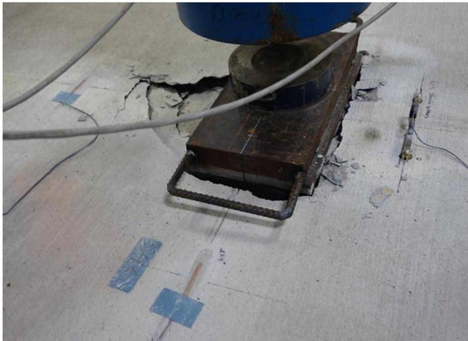
Figure 5.78: Load Case F1 – Failure at load point from top of slab
