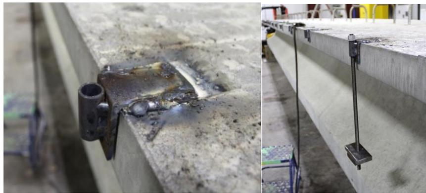
a) Bracket with tube for bolt
