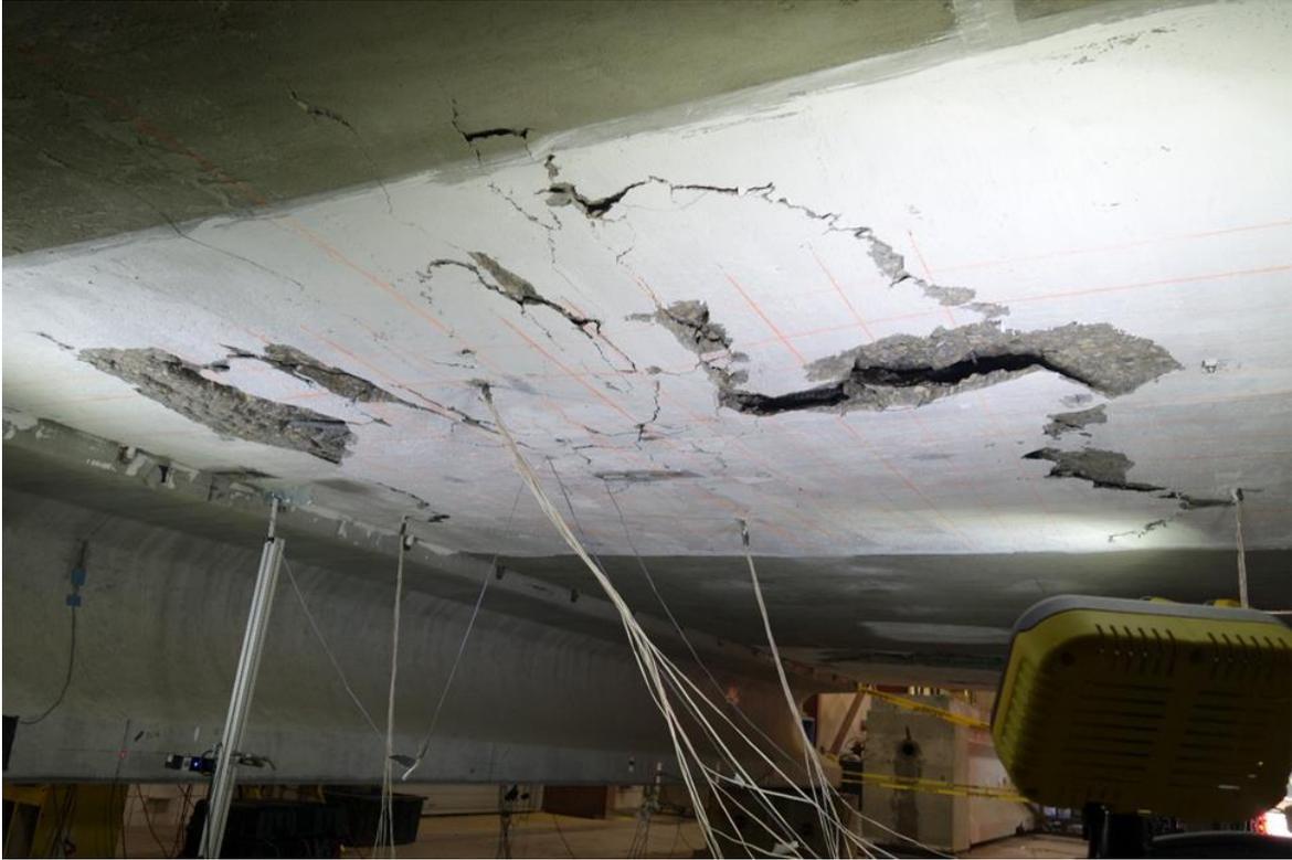
Figure 5.77: Load Case F1 – Failure ellipse area from bottom slab: 87 in. (7.25 ft) x 96 in. (8 ft)
