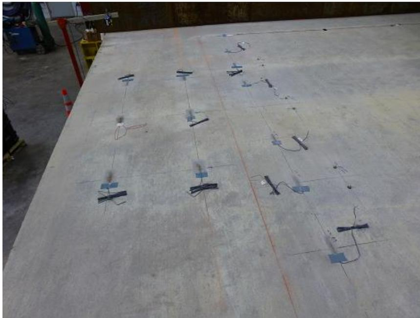
Figure 4.28: S2/F2 surface strain gauges
