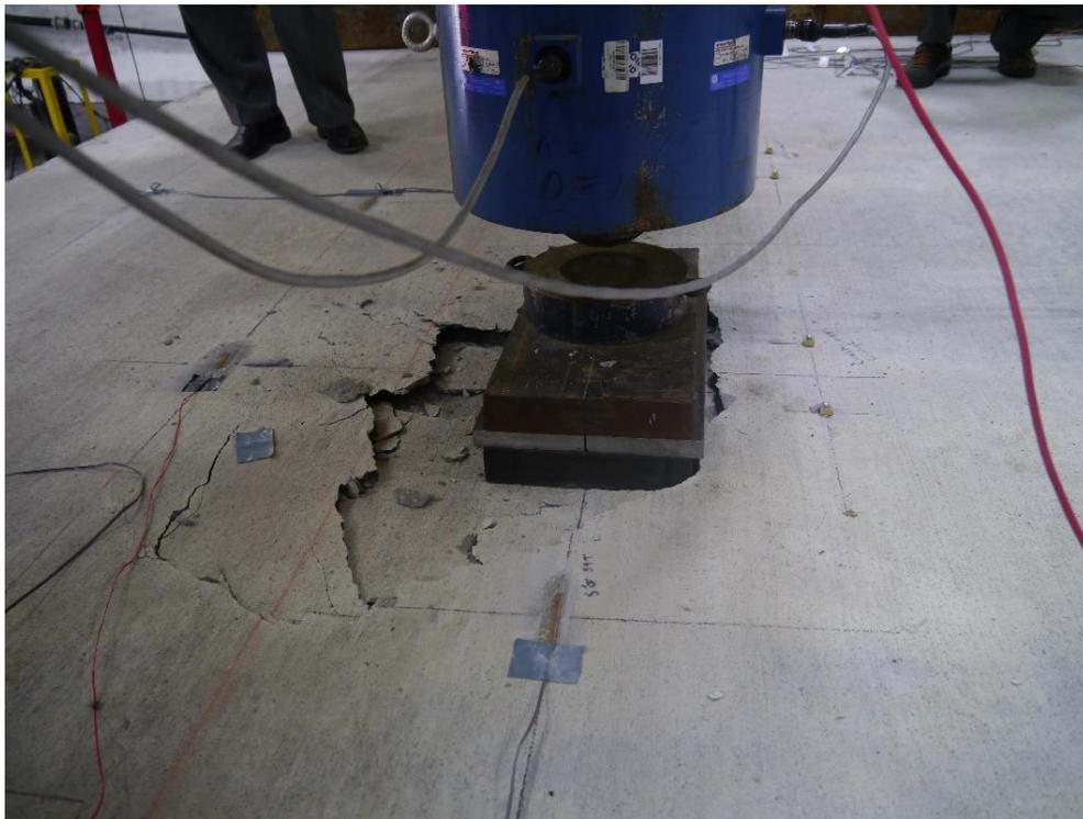
Figure 5.83: Load Case F2 – Failure at the top of slab
